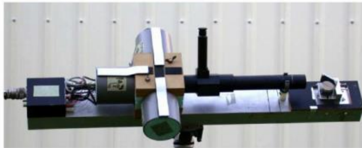
Fig. 3. Top: Components of the Chl fluorescence detector for passive fluorescence measurements in the oxygen absorption band, at 760 nm. 1, reference; 2, target; 3, chopped mirror; 4, field stop; 5, high pass filter; 6, polarization cube; 7, view finder; 8, beam splitter; 9, interference filter (758.5 nm); 10 and 13, lenses; 11 and 14, photodiodes; 12, interference filter (760.5 nm). Bottom: Photograph of the instrument. The length is about 90 cm and the weight 3 kg.
