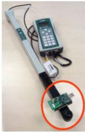
(b) Setting for the direct comparison of WSN versus conventional hardware using a TelosB mounted on the LAI-2200 wand.
