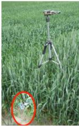
(a) Pair setting with one TelosB on a tripod above and a second one below the canopy (red ellipse) deployed in a wheat field.
